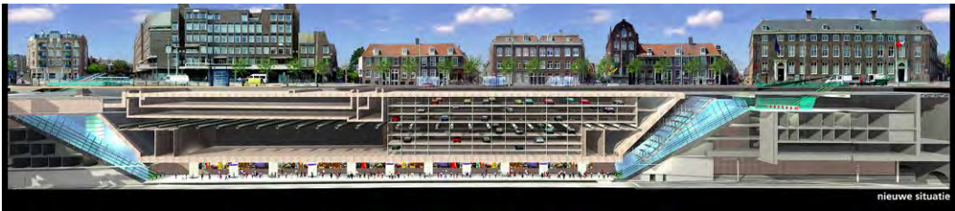
Figure Rendering longitudinal section of Vijzelgracht station
