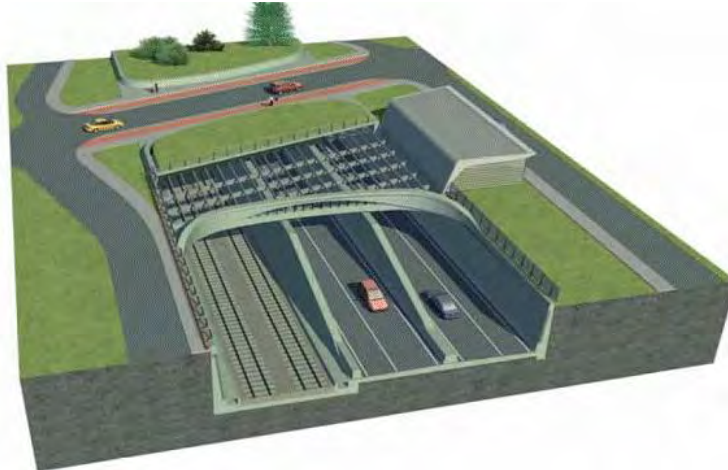
Figure overview road- and raitunnel.
