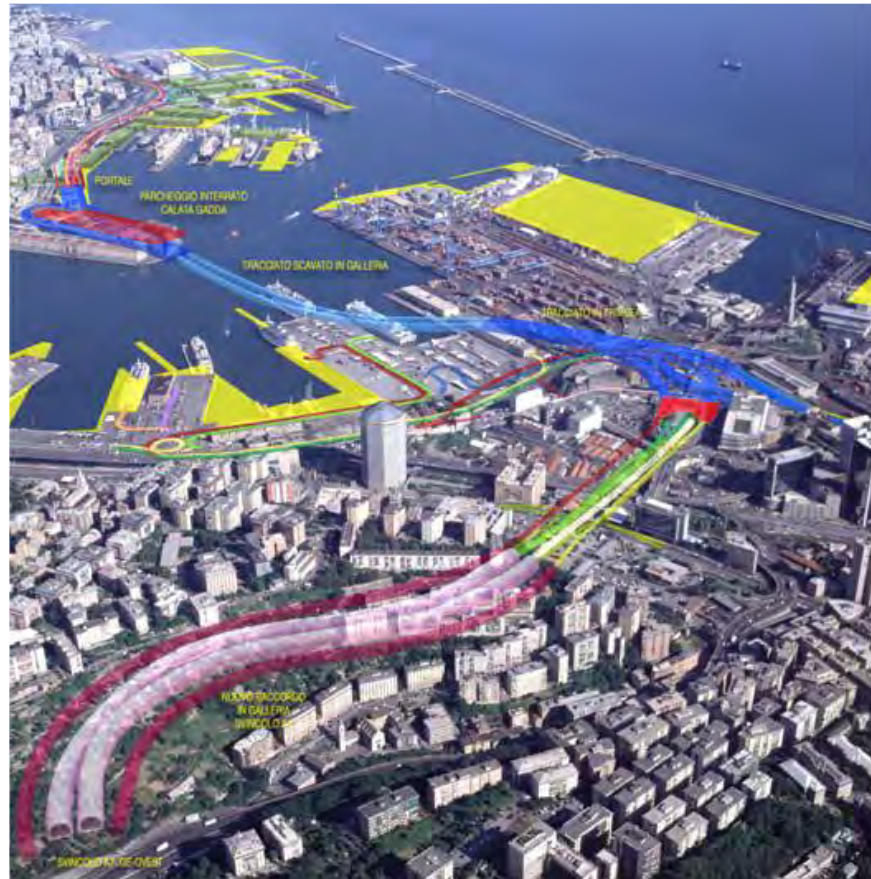
Figure: Tunnel alignment Genoa
