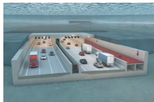
Typical layout immersed tunnel
